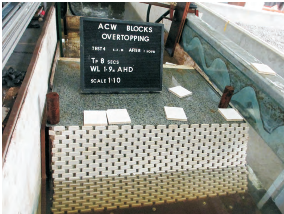
b) Cross-section 1 - placement density 11.9 units/m 2 , WL 1.9m AHD, after 2000 waves, capping dislodged
