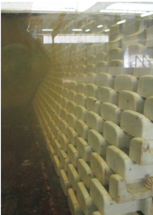
b) Cross-section 2 - placement density 10.8 units/m 2 , WL 1.6m AHD, after 2000 waves, no damage to wall
