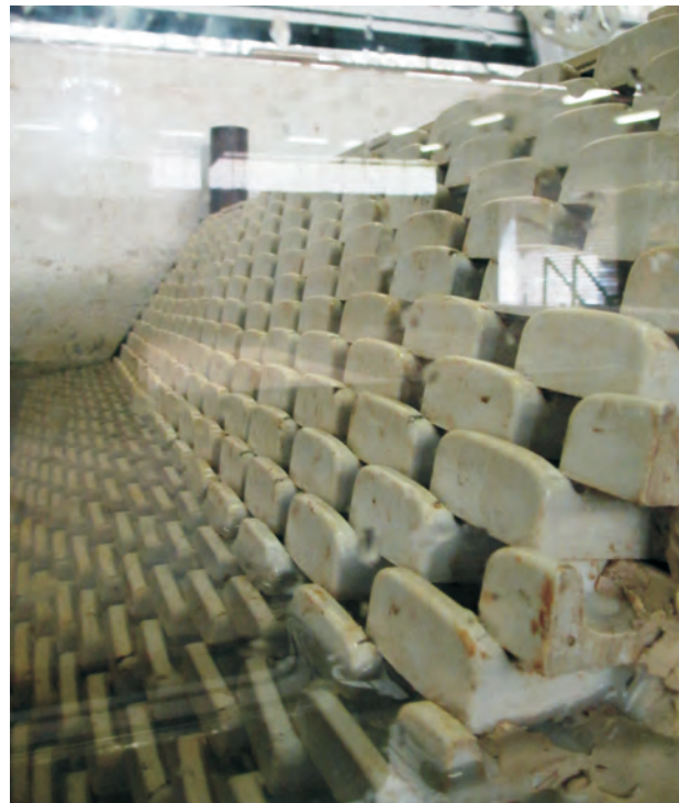
b) Cross-section 2 - placement density 10.8 units/m 2 , WL 1.6m AHD, after 2000 waves, no damage to wall
