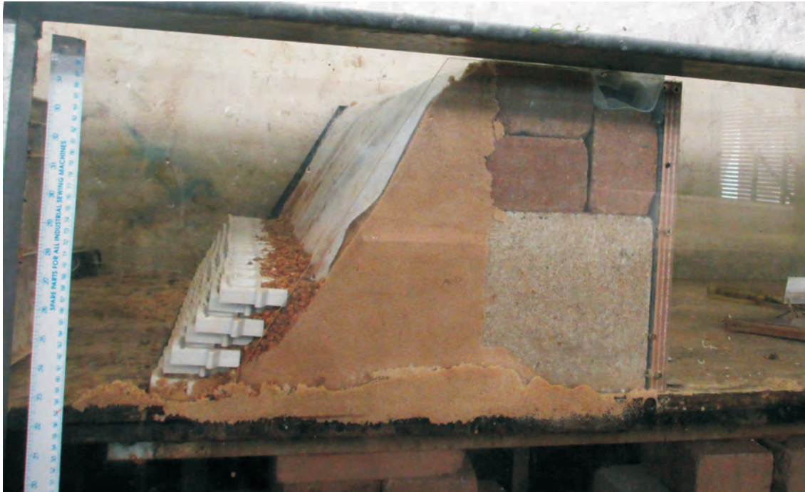
a) Testing possible modes of failure. Cross-section 1 - placement density 11.9 units/m 2 , WL 1.6m AHD, during construction
