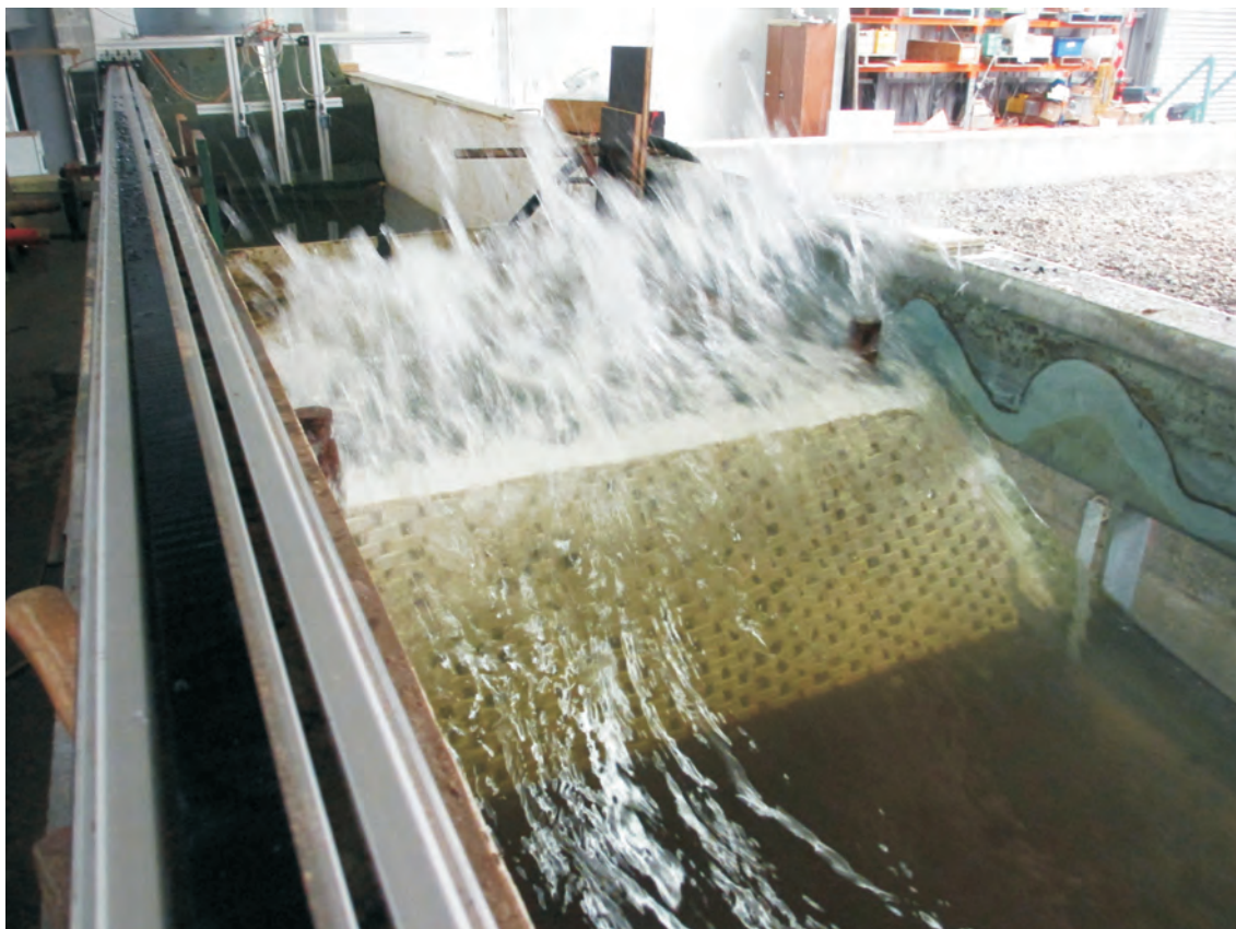
b) Cross-section 1 - placement density 11.9 units/m 2 , WL 1.6m AHD, wave overtopping structure during testing
