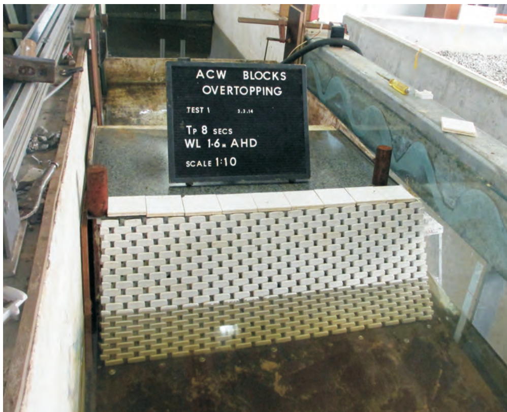
b) Testing possible modes of failure. Cross-section 1 - placement density 11.9 units/m 2 , WL 1.6m AHD, before testing
