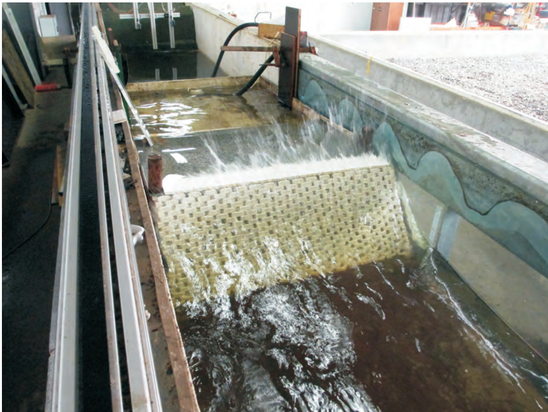
b) Cross-section 1 - placement density 11.9 units/m 2 , WL 1.5m AHD, wave overtopping during testing
