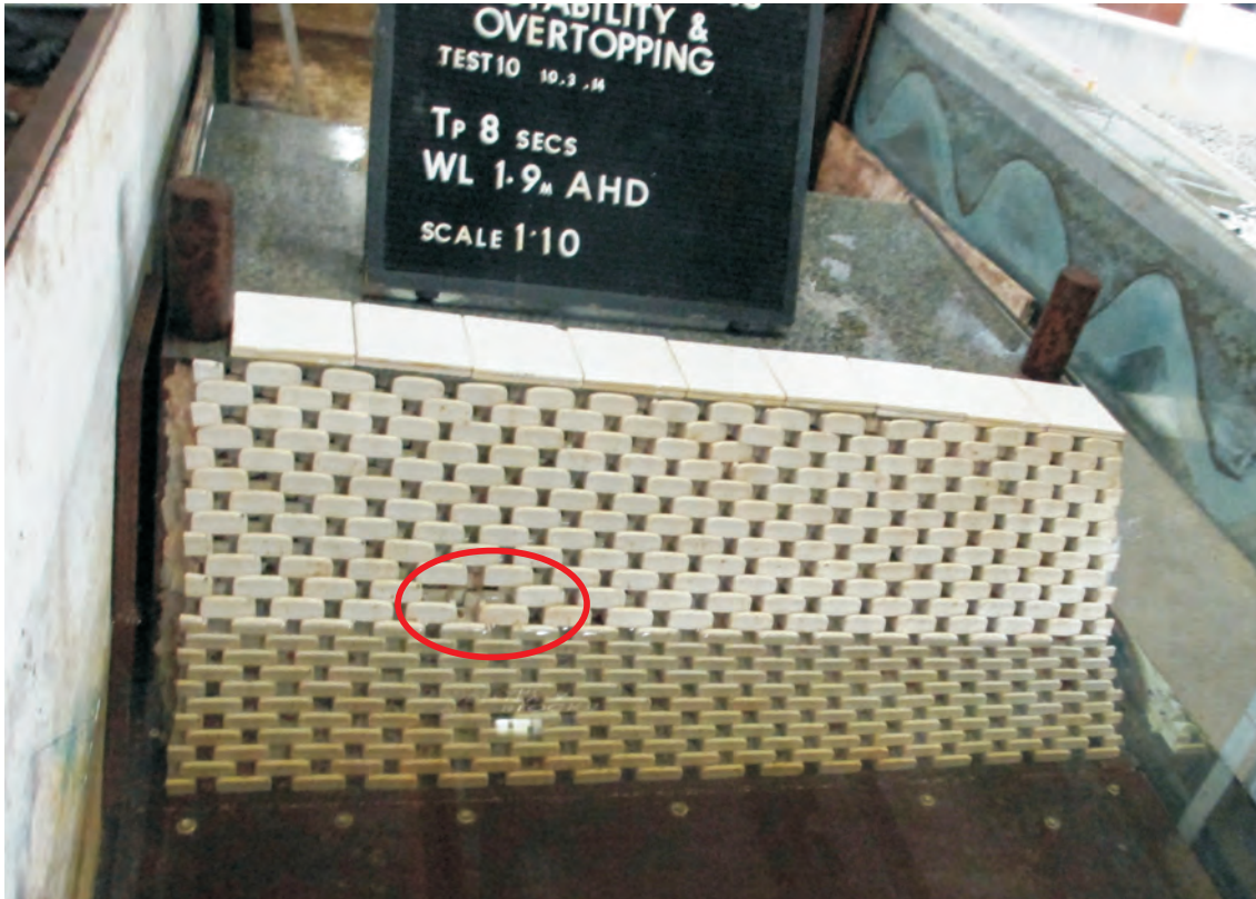
a) Testing possible modes of failure. Cross-section 2 - placement density 10.8 units/m 2 , WL 1.9m AHD, one unit removed, before testing
