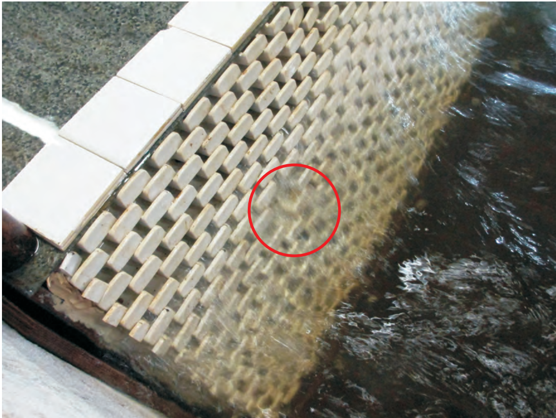
a) Testing possible modes of failure. Cross-section 2 - placement density 10.8 units/m 2 , WL 1.9m AHD, two units removed, during testing
