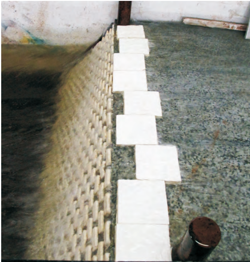
a) Cross-section 2 - placement density 10.8 units/m 2 , WL 1.9m AHD, displacement of capping during testing
