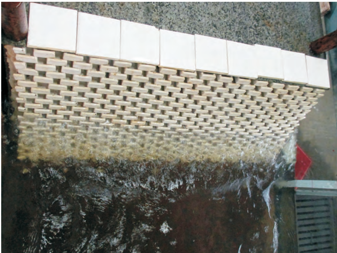
b) Cross-section 2 - placement density 10.8 units/m 2 , WL 1.6m AHD, during testing
