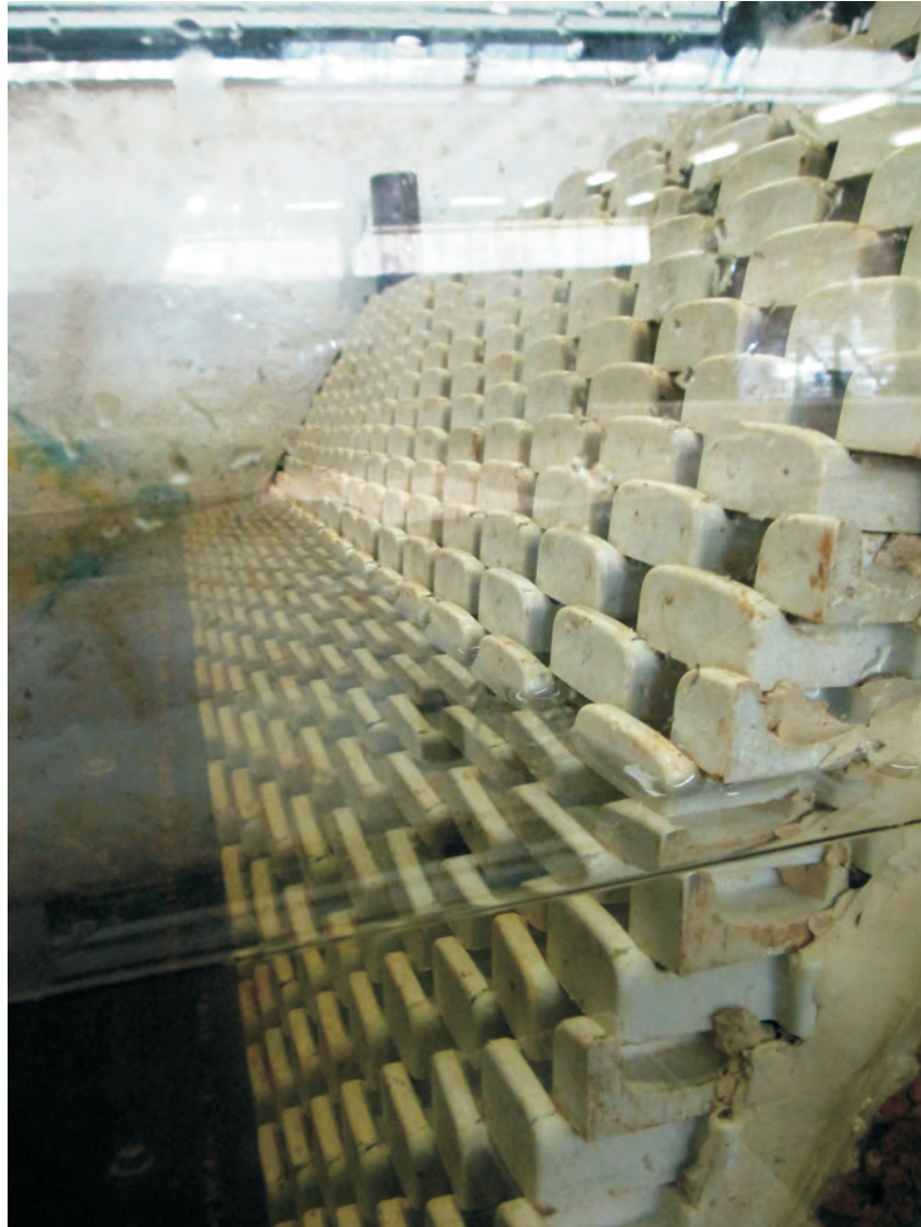
Cross-section 2 - placement density 10.8 units/m 2 , WL 1.9m AHD, after 2000 waves, note displacement of three units resulting in minor damage (<1%), another view
